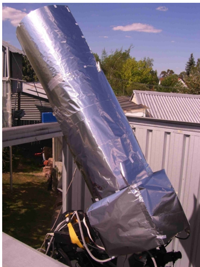
Figure 11. The set-up for the 9th November 2006 Transit of Mercury: Aluminium foil to keep it cool
