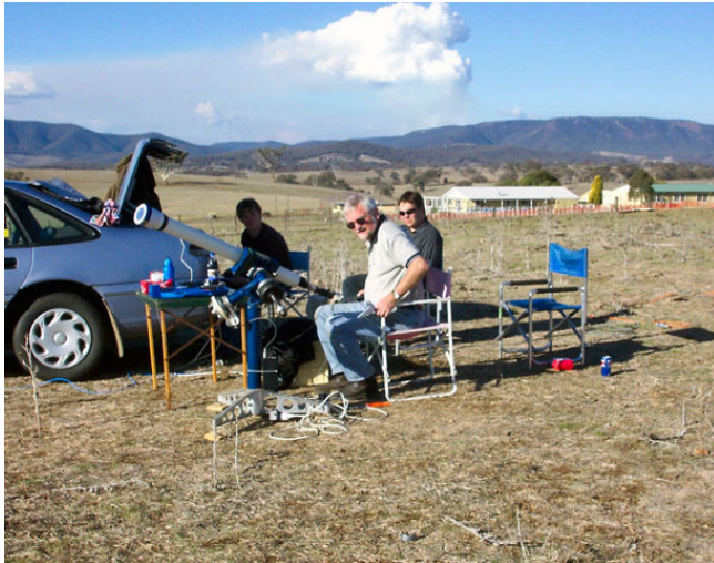
Figure 5. The 3" telescope, camera with the server in the trunk of the car and powered by a 150m cable plugged into a garage power point.
