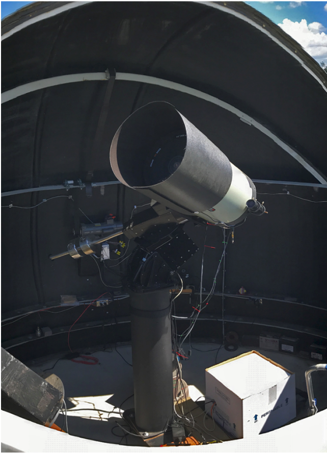
Figure 2. AURT in 2018, picturing the west side of the Astrohaven dome lowered. AURT's Celestron Edge 1400HD 0.36 m f/10 Schmidt-Cassegrain telescope, mounted on a Software Bisque Paramount ME robotic German equatorial mount, forms the core components of the AURT. AURT has been a member of the Skynet telescope network since 2014 and is one of a growing number of Internet-based moderate-aperture telescopes. Photo: Ian Schofield
