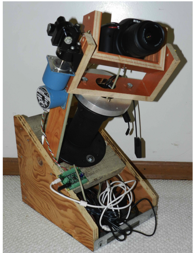
Figure 5. The first version of Algolcam, a tracking DSLR camera fitted with telephoto lens, used for performing photometric measurements on variable stars, with applications in low cost sky surveys, sky monitoring and teaching. Photo: Martin Connors
